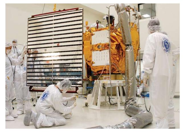
battery. The solar arrays provide energy to the probe and charge the battery; when the spacecraft's orbit carries it behind Mercury and out of the Sun's light, the spacecraft switches to battery power to continue operations.
