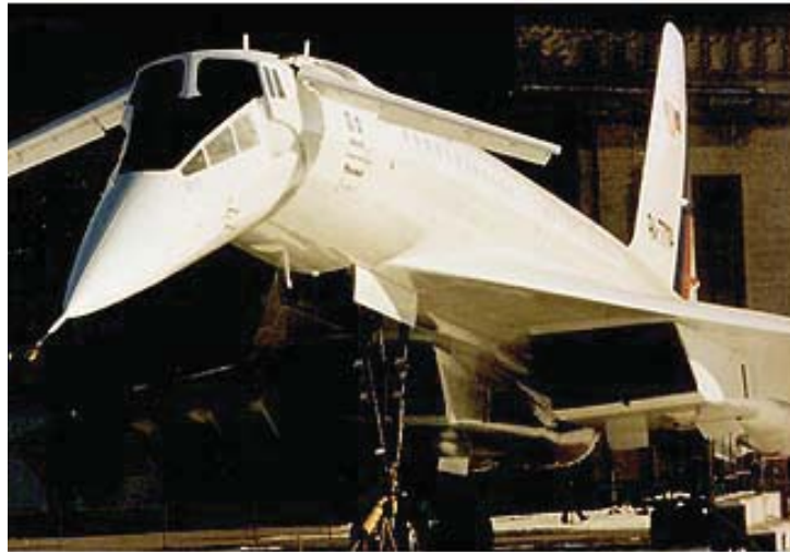
Figure 2: TU-144 Drooped Nose Deployed
