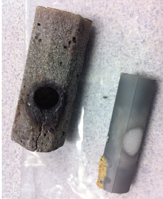
Figure 17. In-coil zirconia ceramic insulator and high-temperature fuel element after high-power testing.
