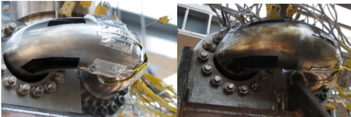
Figure 8: DMLS Duct Before (Left) and After (Right) Hot-Fire Test
