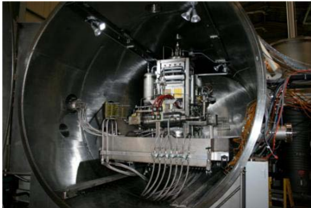
FSP-PTC Stirling & 7 Pin Rx Core Sim Testing
