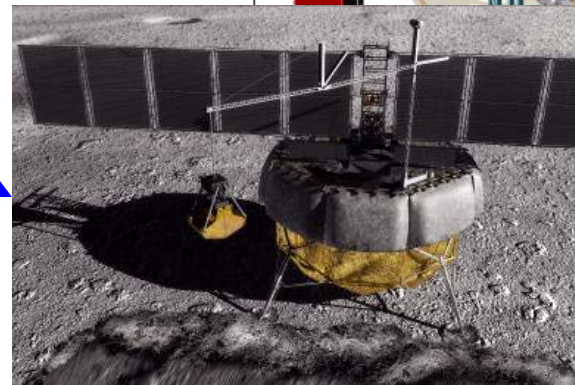
LSS Scenario 5: Lander-Integrated FSP System
