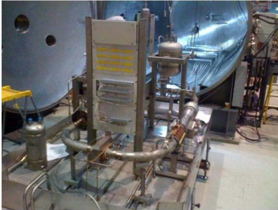
Figure 2. Annular Linear Induction Pump (ALIP) Test Circuit
