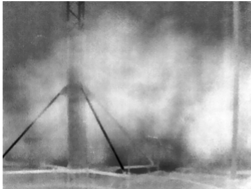
Fig 5. Deleterious effect of wetted exhaust plume on infrared image gathering taken during ASMAT 12
