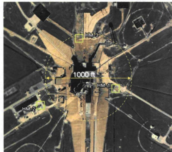
Figure 1. Location of three hail monitor stations, approximately 500 ft from launch pad center.
