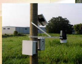
To facilitate analysis of short- and long-term impacts of meteorology, 11 weather stations have been installed across the MSFC property. These data are transmitted by radio to a database for real-time support to the MSFC Facilities Office and the National Weather Service office located in Huntsville.
