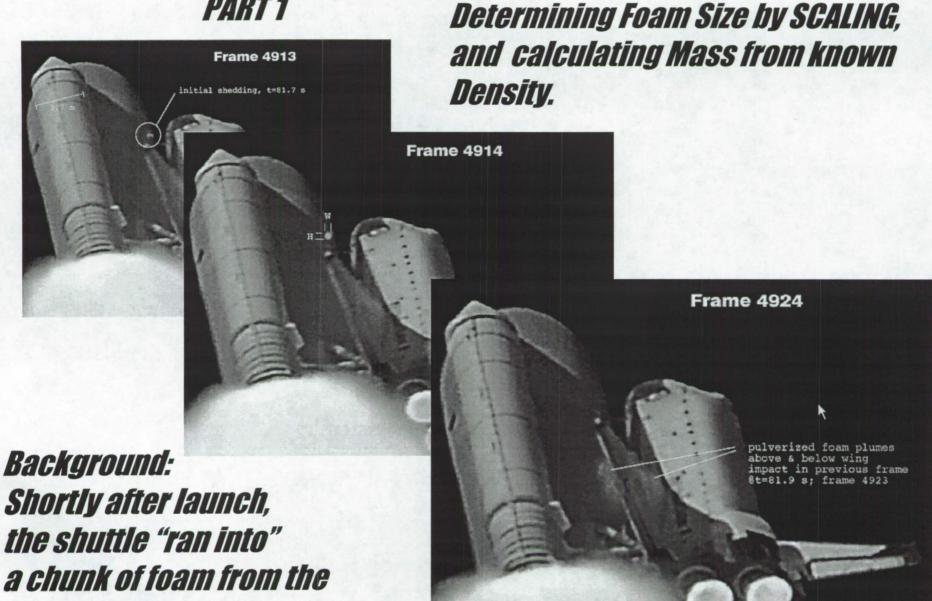
When the Columbia and External Tank were both traveling at 1568 mph, a piece of foam separated from the External Tank.
