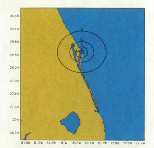
Figure 14. Range of spatial scales FSS was computed over for the 1.33 km nested runs. Circle A represents 5.3 km, B represents 13.3 km, C represents 26.6 km, D represents 53.2 km. The center point of each circle, which represents the grid scale, is located at LC 39A.
