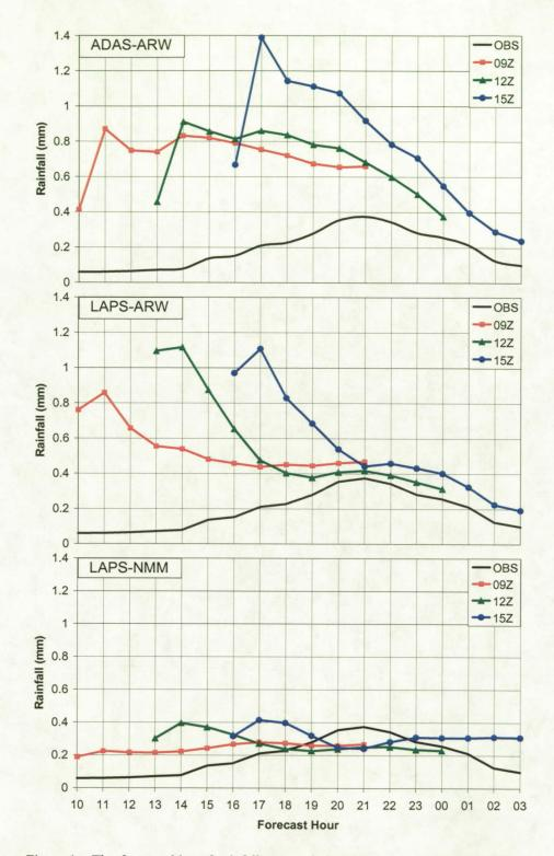
Figure 4. The forecast bias of rainfall accumulation (mm) versus time (UTC) for ADAS-ARW (top), LAPS-ARW (middle), and LAPS-NMM (bottom). The black line is the hourly observed rainfall accumulation averaged over the 4 km domain. The red, green, and blue lines are the averaged forecast rainfall accumulations for all model runs initialized at 0900, 1200, and 1500 UTC, respectively.
