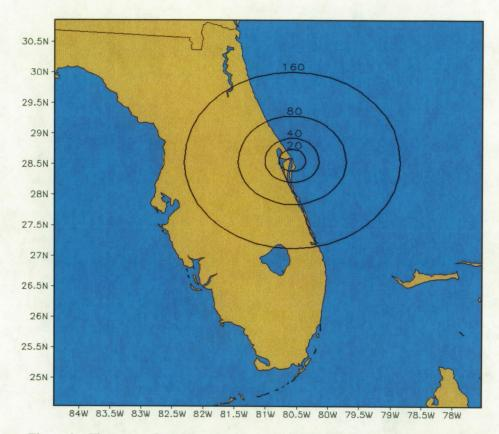
Figure 6. The range of spatial scales for the FSS calculations, starting from the grid scale at 4 km (center point) to 160 km. The center point of each circle is located at LC 39A.
