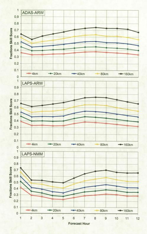
Figure 5. The Fractions Skill Score versus forecast hour for ADAS-ARW (top), LAPS-ARW (middle), and LAPS-NMM (bottom). The colored lines represent model skill on different spatial scales, from the grid scale at 4 km to 160 km. The color legend is on the bottom of each chart.
