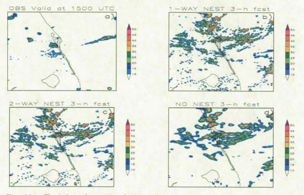
Figure 16. The a) observed composite reflectivity valid at 1500 UTC 17 July 2006 and b) 1-way, c) 2-way, and d) no nesting three-hour forecasts of composite reflectivity initialized at 1200 UTC 17 July 2006.
