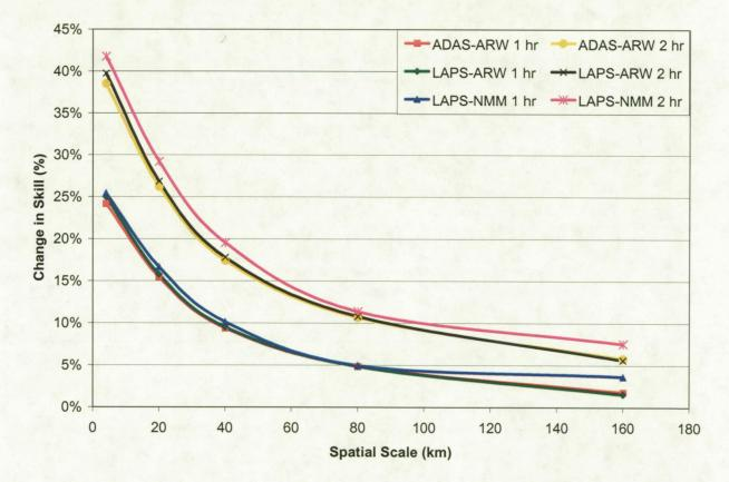
Figure 7. Change in skill when one- and two-hour temporal scales were taken into account for all three WRF model configurations over the range of spatial scales shown in Figure 6. The legend showing the color of each curve for each model and temporal scale combination is in the upper right.
