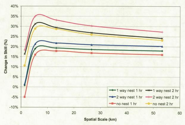
Figure 15. Change in skill when one- and two-hour temporal scales were taken into account for all three LAPS-ARW nesting configurations over the range of spatial scales shown in Figure 14. The legend showing the color of each curve for each model and temporal scale combination is in the lower right.
