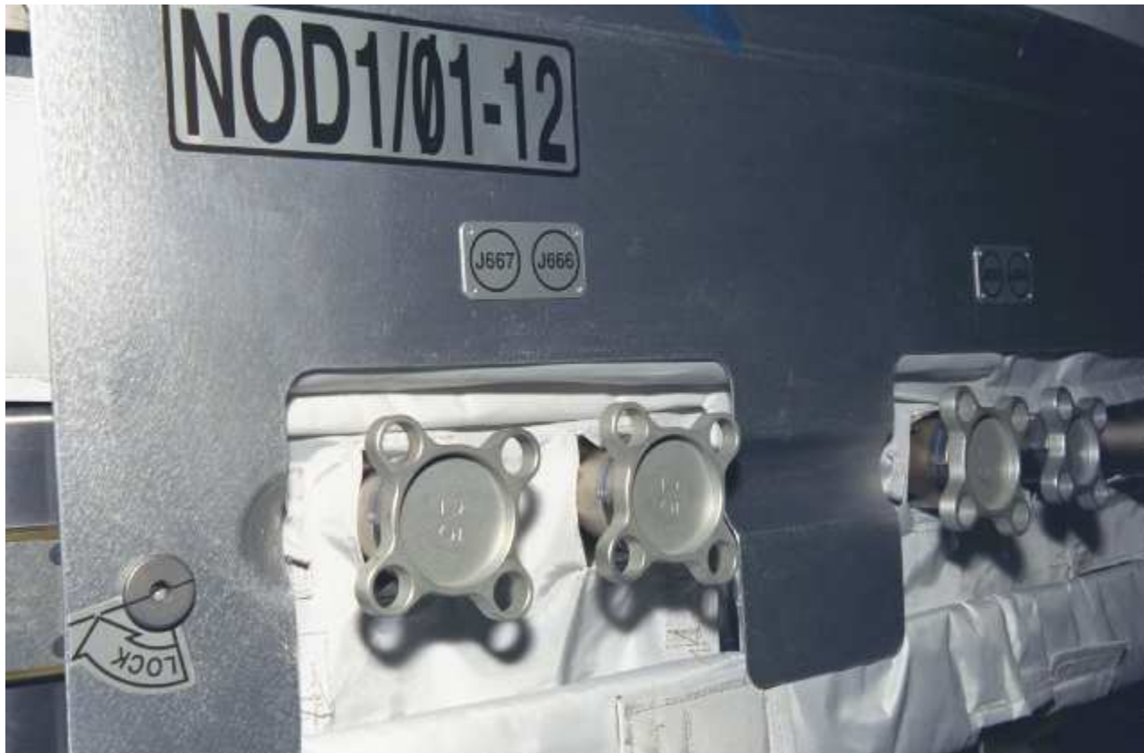
Preflight (closeout) Photo showing anodized foil labels
