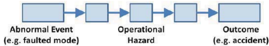
Figure 5: Chain of Events Model Used in DO-312 for Hazard Identification
