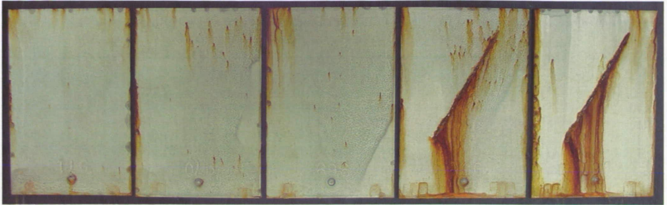
FIGURE 3 – AR-7 after 2000 hours in the salt fog chamber.
