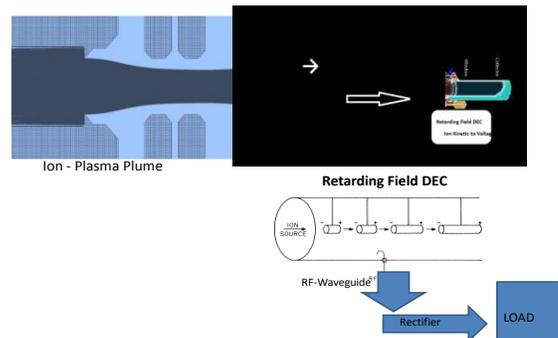
*Ionic injection into TWT- like device Inlet Aperture - Beam collimation, Retarding Field & Gradual braking of ions to limit Bremsstrahlung, Cavity structure w Induced “Ringing”, Waveguide extraction of RF energy from cavity Rectification of RF for power conversion & distribution*
