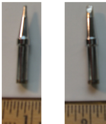
Figure 7.—Soldering iron tips provided in CRE-1 Tool Kit: 1/32 in. (left) and 1/8 in. (right).
