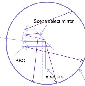
Optical modeling used to predict emissivity performance
