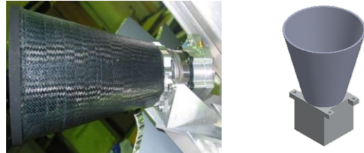
Fig. 11: Surrey star tracker 6 (left) and emulated star tracker (right).
