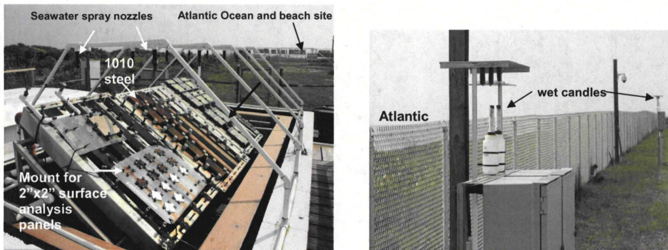
Figure 2: Alternating Seawater Spray system with exposure panels, and modification for panels used for surface analysis (left). Wet candles exposed to KSC beachside atmospheric conditions and used to measure chloride concentration per month (right).
