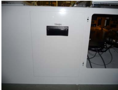
Figure 10. Trash compartment (view from aisle).
