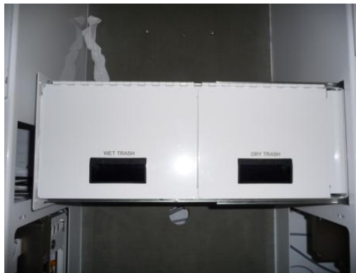
Figure 11. Trash compartment (extended into aisle).
