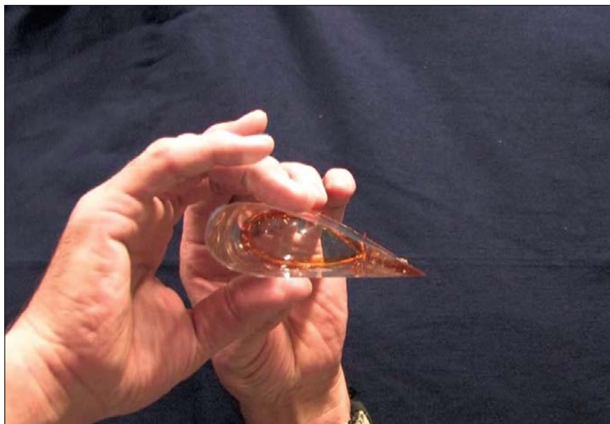
Figure 2. Top View of the 0 G Cup showing the cup profile and the liquid channel at the rim.
