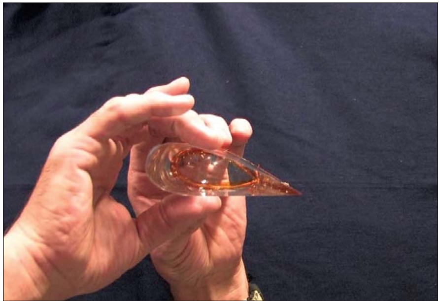
Figure 2. Top View of the 0 G Cup showing the cup profile and the liquid channel at the rim.
