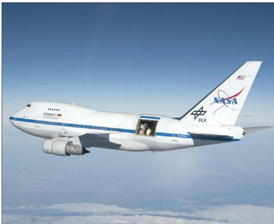
Photo of 747SP SOFIA Airplane undergoing tests in an open-door configuration.
