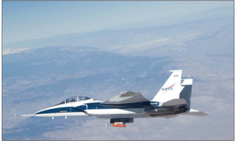
The NASA Dryden F-15B research test bed with Propulsion Flight Test Fixture pylon and Rake Airflow Gage Experiment rake during flight test.
