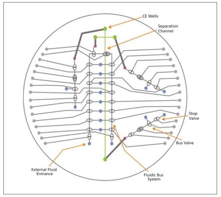
Shown here is the **Layout of a Chemistry "Circuit"** designed for the purpose of performing automated analyses of amino acids. Experiments have been performed in which a sample of amino acids is placed on the surface of a chip. All subsequent sample handling processes are performed by the microfluidic circuit shown here.
