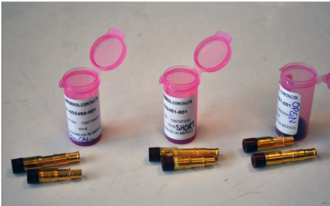
Figure 6.—Open, short, and wide-load terminations for 150- \Omega vector network analyzer (VNA) calibration.
