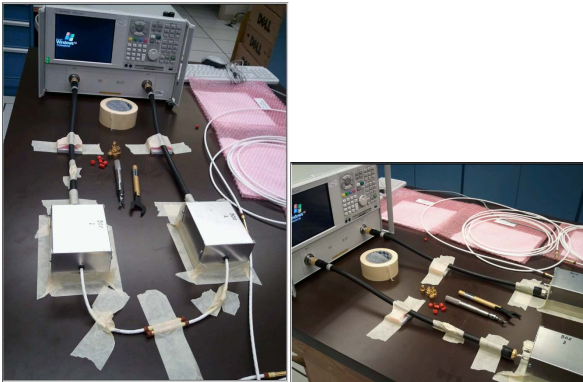
Figure 5.—Typical calibration with balun Box1 and Box2 connected via pigtail cables and terminated in 150- \Omega , open, or short load.
