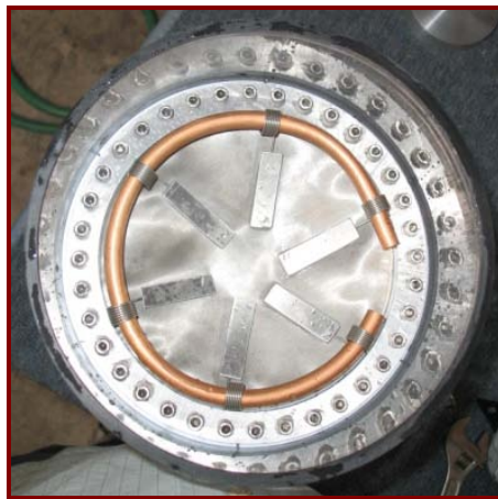
Figure 15. Initial Spring Loading Mechanism Below Screen
