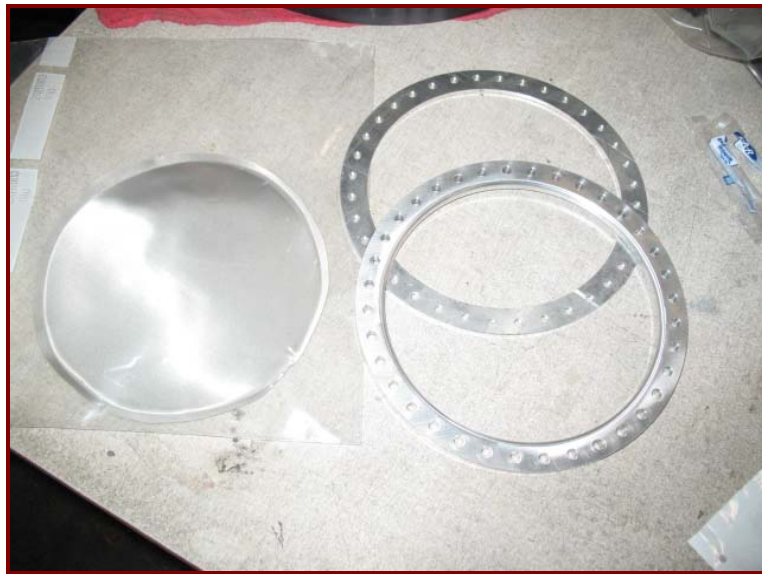
Figure 11. Inner retaining ring and PMD Screen
