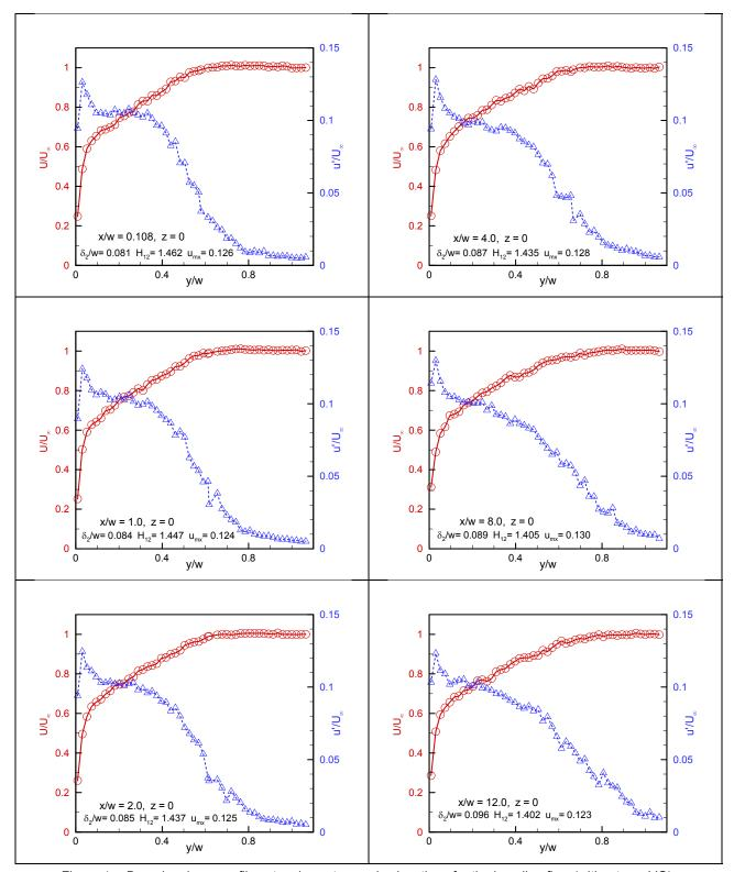
Figure 4.—Boundary layer profiles at various streamwise locations for the baseline flow (without any VG).
