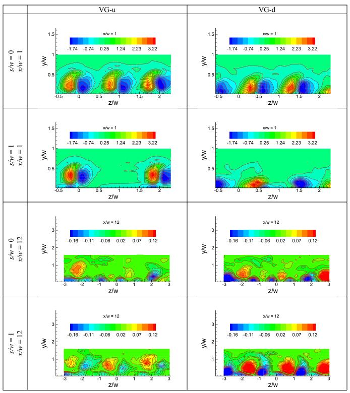
Figure 17.—Comparison of streamwise vorticity at x/w = 1 and 12 for s/w = 0 and 1, as indicated. Left column for 'upwash' orientation (VG-u) and right column for 'downwash' orientation of vortex generator (VG-d).
