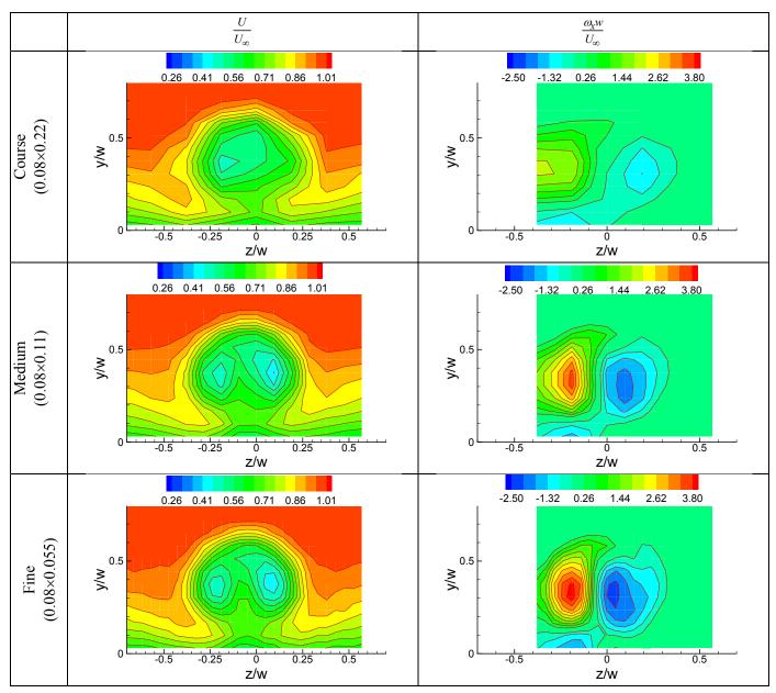
Figure 6.—Effect of measurement grid resolution on mean velocity and streamwise vorticity distribution at x/w = 1; data are for a single VG with 'upwash' orientation (VG-u).
