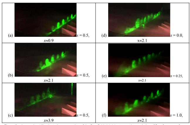
Figure 3.—Laser-sheet illuminated cross-section of the flow field. (a)-(c): streamwise evolution of flow for array of 5 VG with spacing s/w = 0.5; (d)-(f): flow at a fixed streamwise location for array of 5 VG with different spacing.
