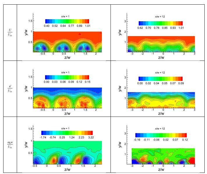
Figure 13.—Mean velocity, turbulence intensity and streamwise vorticity distributions at two x-locations for the array of 5 VG-d with spacing s/w = 0; VG-d is VG with reversed orientation producing a 'downwash' directly behind.
