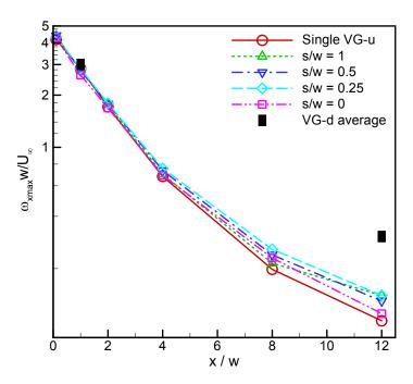
Figure 18.—Peak streamwise vorticity versus x for different VG cases as indicated;  $\omega_{xmax}$  is the average of absolute peak values in the two components of the vortex pair.
