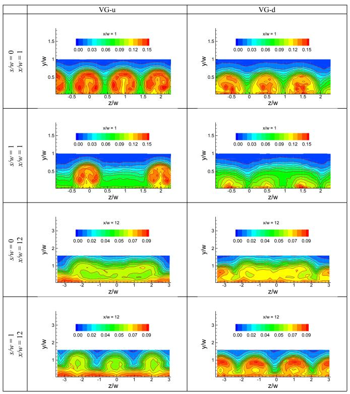
Figure 16.—Comparison of turbulence intensity at x/w = 1 and 12 for s/w = 0 and 1, as indicated. Left column for 'upwash' orientation (VG-u) and right column for 'downwash' orientation of vortex generator (VG-d).
