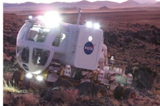
Fig. 3. Space Exploration Vehicle (SEV). Previously known as Chariot or the Lunar Electric Rover (LER).
