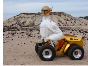
Fig. 2. Centaur 1 robot. Consists of a Robonaut 1 upper body with a four-wheeled lower body.
