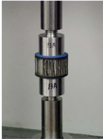
Figure 9: Flatwise Tension Geometry used for Disbond Investigation
