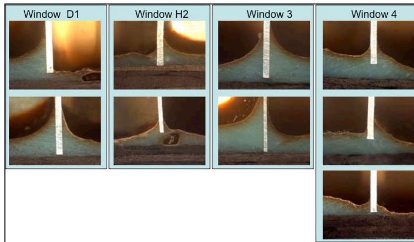
Figure 16: Fillet Quality from Samples Extracted from the Four Windows
