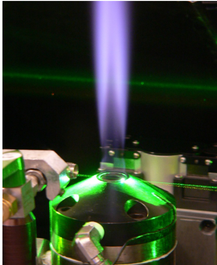
Figure 7-1: Visible image of the laboratory-scale supersonic combustor free jet
