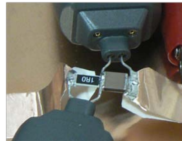
Figure 9. Chip capacitor - chip resistor arrangement
