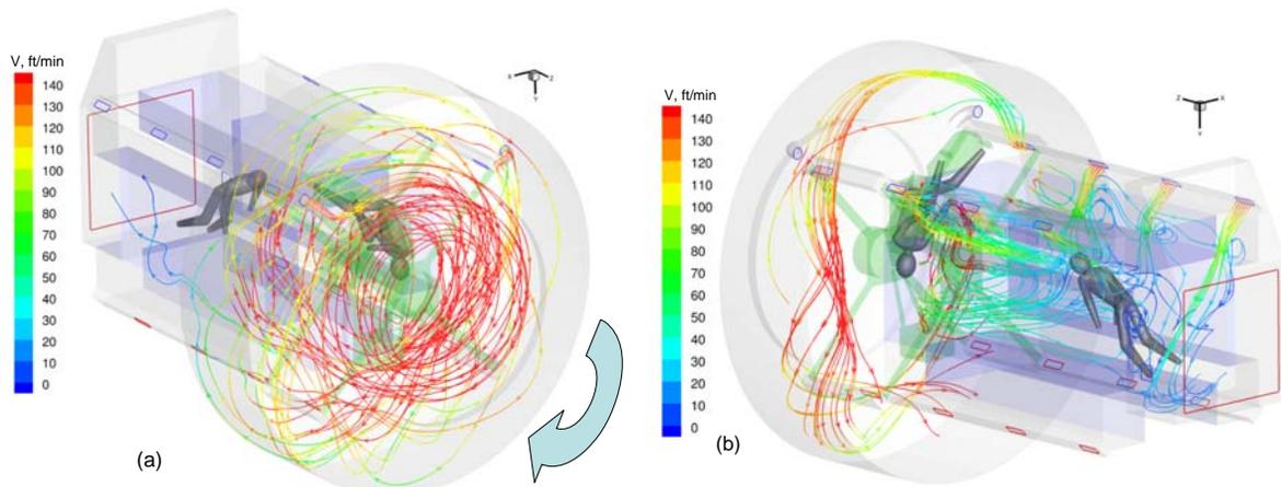
**Figure 3. Pathlines colored with velocity magnitude for an instant when the crew is exercising, Case 2: (a) issued from the PMM endcone diffusers; (b) issued from the PMM main air supply diffusers.**
