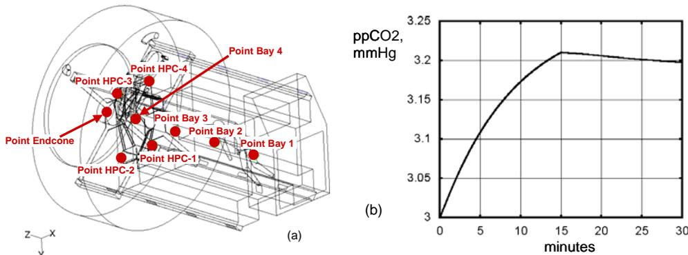
**Figure 6. (a) Monitoring points positions. (b) Volume-averaged carbon dioxide concentration evolution.**
