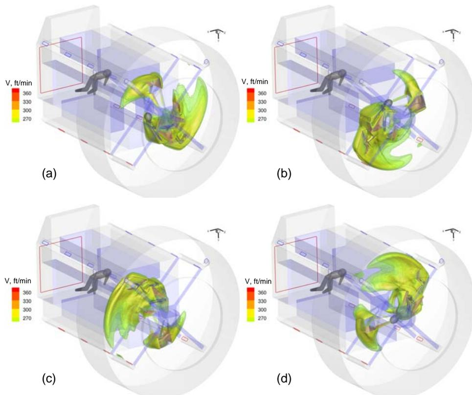
**Figure 4. Instantaneous isosurfaces of air velocities computed for Case 2 presented for the instants of (a)  $T_0$ , (b)  $T_0 + 0.5$  s, (c)  $T_0 + 1$  s, (d)  $T_0 + 1.5$  s.**
