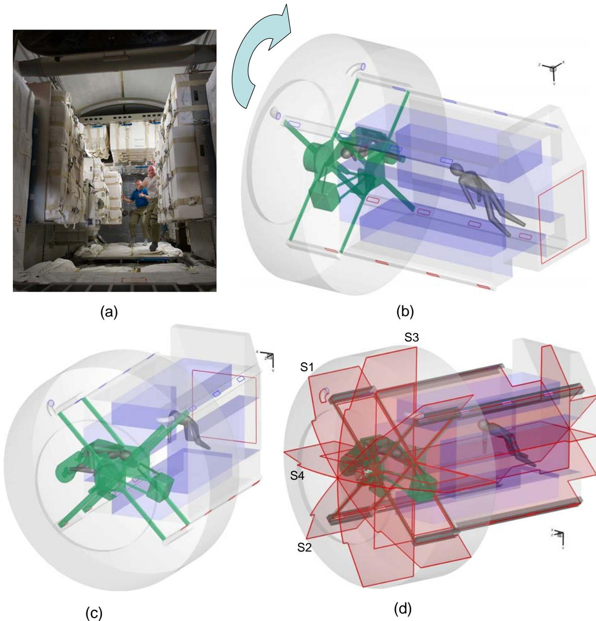
**Figure 1. (a) Interior of PMM after its installation in ISS<sup>7</sup>; (b-d) views of the geometry model used for CFD study of CO<sub>2</sub> transport in PMM when crew is exercising on HPC.**
