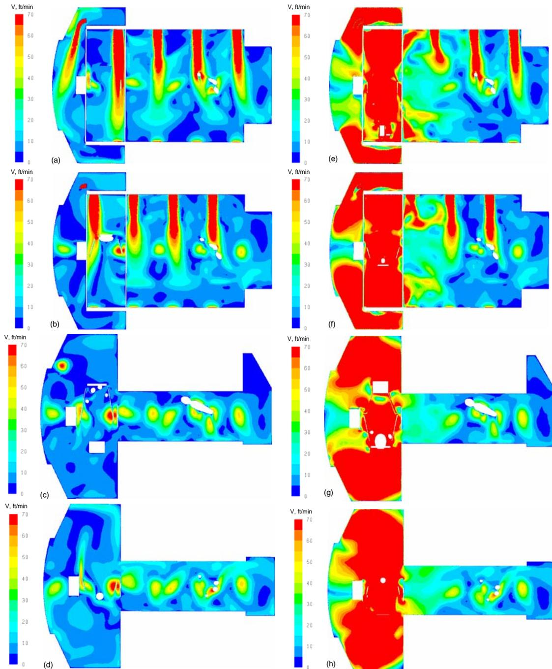
**Figure 2. PMM velocity magnitude distributions computed for (left) Case 1 without rotation and (right) Case 2 with rotating HPC and ECLOID in Bay 4: (a,e) diagonal slice S1; (b,f) diagonal slice S2; (c,g) slice  $x=0$ ; (d,h) slice  $y=0$ .**
