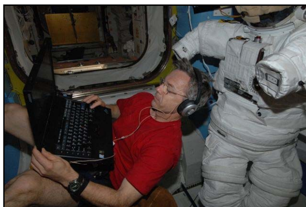
Figure 1. A crewmember performing the OOHA test during Expedition #20. Insert ear monitors are being worn underneath the visible Bose active noise reduction headset, as the crewmember uses a software program on his computer to assess his hearing sensitivity.
