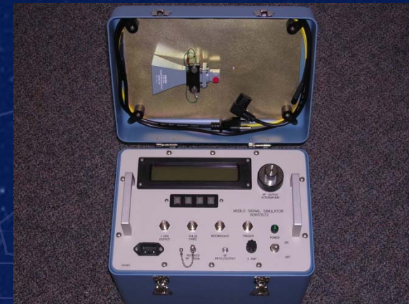
Microwave Scanning Beam Landing System (MSBLS) signal simulator
