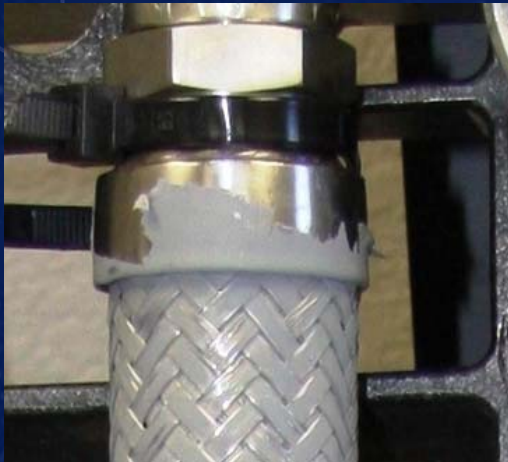
Adhesion problems of GE 3404 on flex hose.
