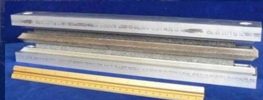
Internal construction of subscale heat exchanger is two pieces of aluminum foam sandwiched between aluminum plates.
