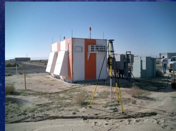
Microwave Scanning Beam Landing System (MSBLS) signal simulator
