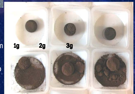
JSC-1A heated to 1100° C for 30 minutes in air
