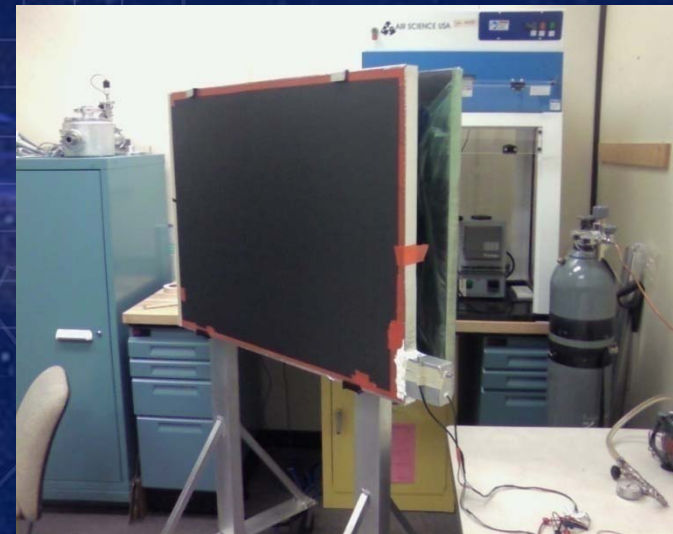
Test setup with Graphite Epoxy Aluminum Honeycomb composite panels built by ATK to be similar to proposed Ares V payload fairings
