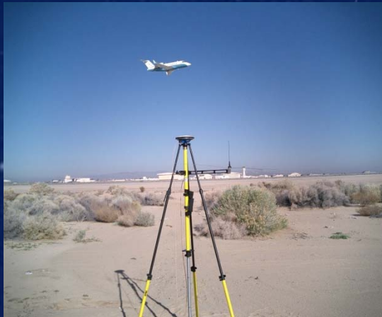
Differential GPS reference station
