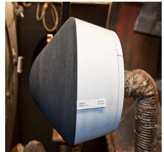
Post-Test Charred PICA Heatshield
