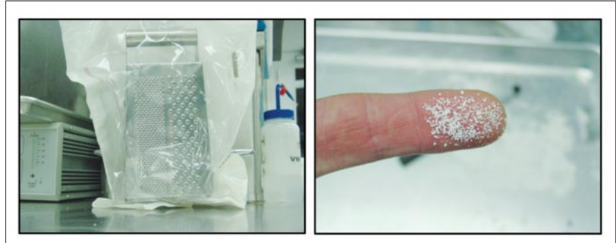
The Box Grater (left), and the size of Cured Paint Particles that were generated upon grating (right).
