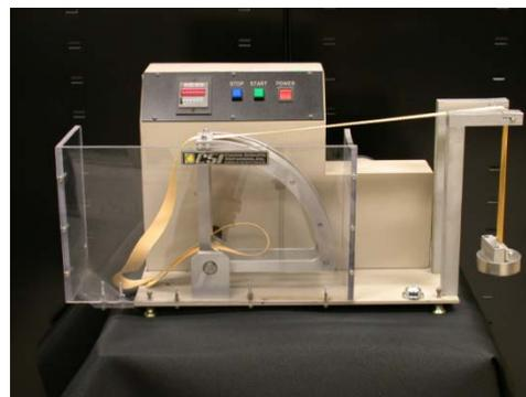
The Multimotion Abrasion Pilling Tester measures the pilling tendency of woven and knitted fibrous structures by subjecting a specimen to multimotion abrasion cycles. Properties that can be studied include shedding tendencies, resistance to abrasion, and the tendency to acquire shine or gloss. The applicable test standard includes ASTM D3511.
