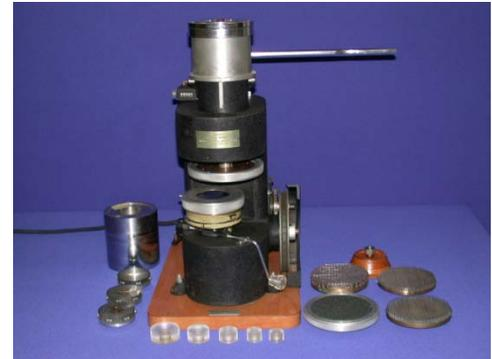
The Wyco Precision Wear Tester is an abrasion machine with an oscillating drum mechanism. It subjects the test specimens to known conditions of pressure, tension, and abrasion action. It can be used with various abrasive surfaces such as sandpaper, wire mesh, leather, and cloth. The abrasion resistance of the specimen is assessed by measuring the number of cycles to failure, reduction of strength, or visual changes. The applicable test standard includes ASTM D4157.
