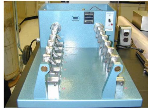
The M.I.T. Folding Endurance Tester is used to estimate the ability of paper or textile to withstand repeated bending, folding, and creasing. It could also be used to measure the deterioration of paper upon aging. The applicable test standards include ASTM D2176 and ISO 5626.
