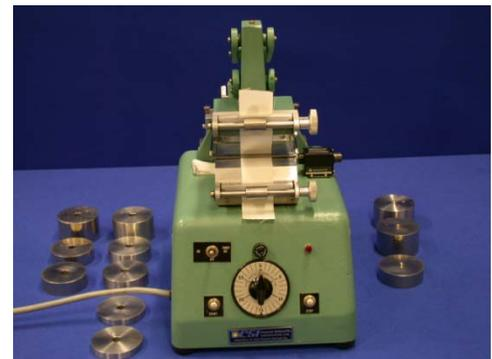
The CSI Stoll Quartermaster Universal Wear Tester is an inflated diaphragm abrasion tester designed to assess the wear resistance of textile or other fibrous structures. A test specimen is rubbed either unidirectionally or multidirectionally against a specified abrasive surface. The specimen is held in a fixed position and supported by an inflated rubber diaphragm that is held under constant pressure. The applicable test standard includes ASTM D3886.
