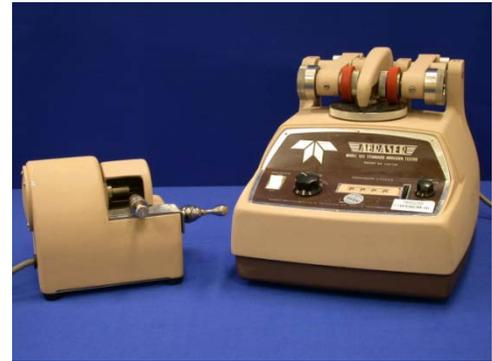
The Schiefer Abrasion Testing Machine applies a uniform abrasive action on the entire surface of a test specimen. It is ideal for evaluating fabric construction that has various fiber blends and finishing treatments. The applicable test standard includes ASTM D4158.
