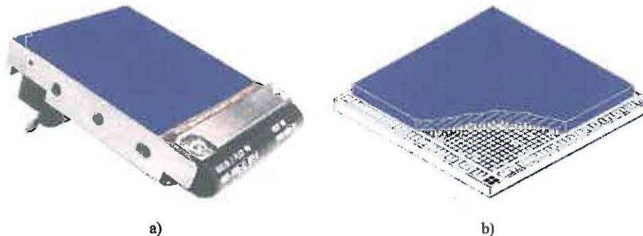
FIG. 2. a) This figure shows a NIRSpect H2RG detector array. The H2RGs used by NIRCcam and FGS/NIRISS differ only in the mechanical packaging. The photosensitive area measures about 36.72 \times 36.72 \text{ mm}^2 . The H2RG has 2040 \times 2040 photosensitive HgCdTe pixels that are surrounded on all sides by a four pixel wide border of “reference pixels.” b) Indium bump bonds are used to join the HgCdTe detector array to the silicon readout integrated circuit (ROIC).
