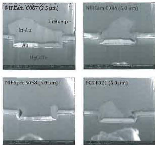
FIG. 11. Scanning Electron Microscopy images of pixels from a Process Evaluation Chip of NIRCcam, NIRSspec, and FGS flight detectors. The presence of In-Au intermetallics from the breakdown of the barrier layer, as indicated by lighter shading in the In and Au layers, is present in all of the images.
