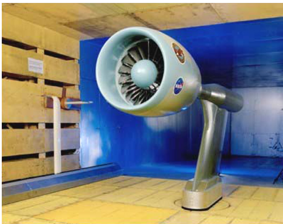
Figure 5.1.—The 22-in.-diameter Advanced Ducted Propulsor (ADP) Fan 1 installed in the NASA 9- by 15-Foot Low-Speed Wind Tunnel. Traversing microphone (located on white stand) is visible to left of model. Microphone moves on track parallel with axis of fan.
