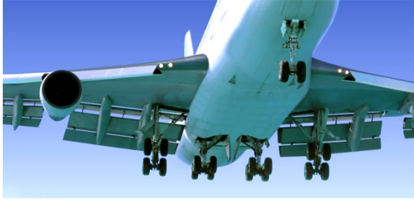
Figure 4.1.—Boeing 747 aircraft in landing configuration. Four main landing gear, nose landing gear, leading-edge slats and triple-slotted, trailing-edge flaps are deployed during airport approach.
