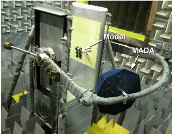
Figure 4.16.—Boeing 777 main gear model assembly mounted in Quiet Flow Facility (QFF) for lateral “sideline” measurements by Medium Aperture Directional Array (MADA) microphones.
