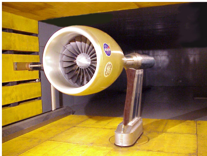
Figure 5.3.—The 22-in.-diameter Source Diagnostic Test (SDT) fan installed in NASA 9- by 15-Foot Low-Speed Wind Tunnel.
