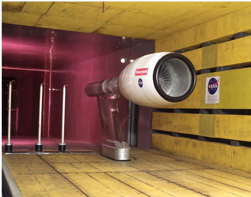
Figure 5.5.—The 22-in.-diameter Quiet High-Speed Fan 2 (QHSF 2) fan installed in NASA 9- by 15-Foot Low-Speed Wind Tunnel.
