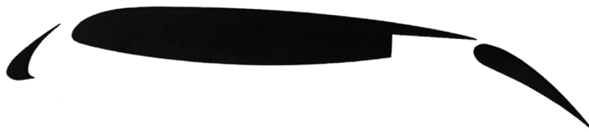
Figure 4.45.—Model three-element 30P/30N high-lift aircraft wing system.
