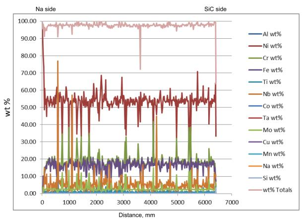
Figure 22.—Wavelength dispersive spectroscopy (WDS) quantitative line scan of major elements for the entire thickness of test Sample 1A.
