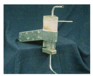
1/10<sup>th</sup> Segment Heat Pipe w/Gas-gap Calorimeter.
