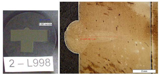
Electron beam weld penetration of 3.5 mm
