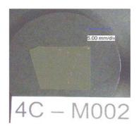
Electron beam weld penetration of 4.5 mm. Unwelded joint section of approximately 1 mm.
