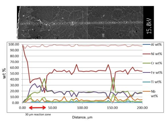
Figure 27.—Electron microprobe image and wavelength dispersive spectroscopy (WDS) quantitative line scan of major elements for test Sample 5A near the sodium (inner) surface.
