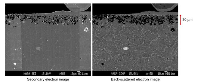
Figure 19.—Electron microprobe images showing the 30  $\mu m$  affected region observed on the sodium (inner) side of Sample 1A.
