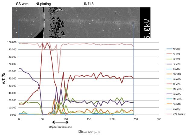
Figure 20.—Electron microprobe image and wavelength dispersive spectroscopy (WDS) quantitative line scan of major elements for test Sample 1A near the sodium (inner) surface.
