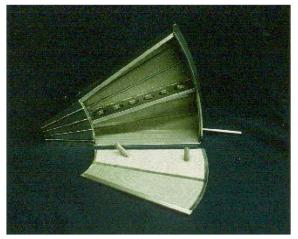
1/10<sup>th</sup> Segment Heat Pipe, Top Plate Removed.
