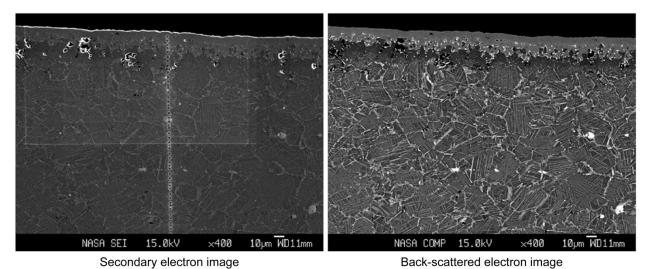
Figure 25.—Electron microprobe images of the sodium (inner) side of Sample 5A.
