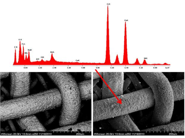
Figure 36.—Concentration chart of major elements and electron microprobe images of the course stainless steel screen from Sample 5A.
