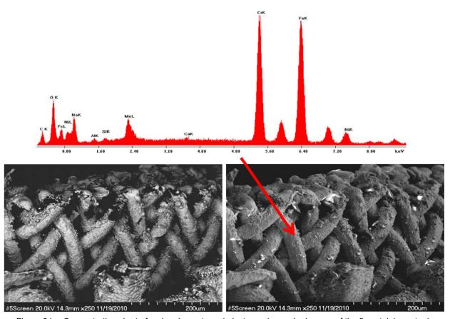
Figure 34.—Concentration chart of major elements and electron microprobe images of the fine stainless steel screen from Sample 5A.
