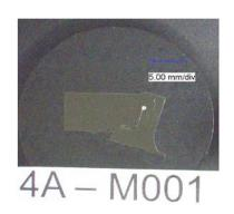
Electron beam weld penetration of 5.4 mm. Only 2 mm of joint welded due to misalignment of joint to electron beam weld.
