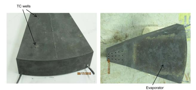
Figure 3.—Heat pipe at the end of life testing.
