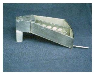
1/10<sup>th</sup> Segment Heat Pipe, Operating Orientation.
