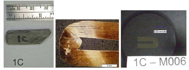
Figure 9.—Sample preparation steps for 1C.
