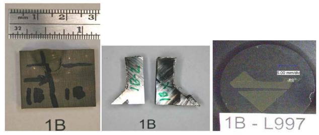
Figure 8.—Sample preparation steps for 1B.
