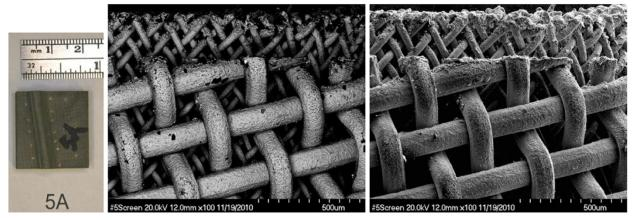
Figure 33.—Electron microprobe images of fine and course stainless steel screens from Sample 5A.
