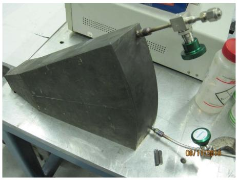
Figure 4.—Vessels attached to heat pipe fill ports.
