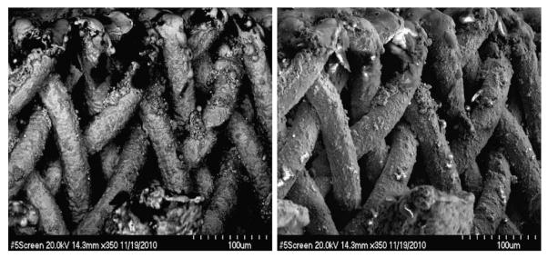
Figure 35.—Higher magnification electron microprobe images of the fine stainless steel screen from Sample 5A.
