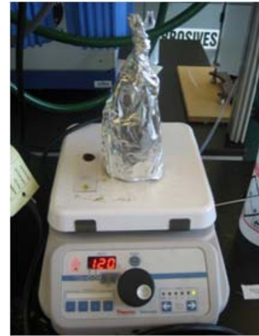
(c) The clamping fixture heated for 10 minutes at 120°C.
