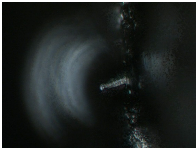
Figure 15. Flight mixed solder board CH4 DIP, lead 2 of 14, 18- \mu m whisker.
