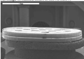
The stacked filters were found to remain bonded after cryogenic thermal cycling. Furthermore, the size of the passband is larger for the stacked filters; a representative transmittance curve is presented below:
