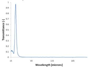
The curve exhibits a high peak transmittance at the design frequency, which, guided by electromagnetic modeling software, is 28.5 microns. Furthermore, the roll-off is sharp and the out-of-band rejection is high. The feature exhibited at low wavelength is a consequence of scattering into higher order modes.
