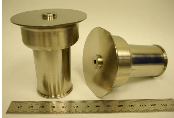
Figure 3.—ASC-E2 production heater head assemblies.
