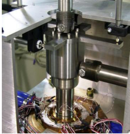
Figure 4.—ASC–E2 heater head installed in the lateral load test setup.
