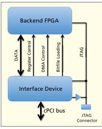
The **cPCI** Interface is a common interface between the cPCI bus and the backend FPGA. It is implemented as a separate interface device on the cPCI bus.
