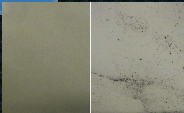
Spherical ZrO 2 Powder (-53/+45 μm) before and after fluidization at room temperature
