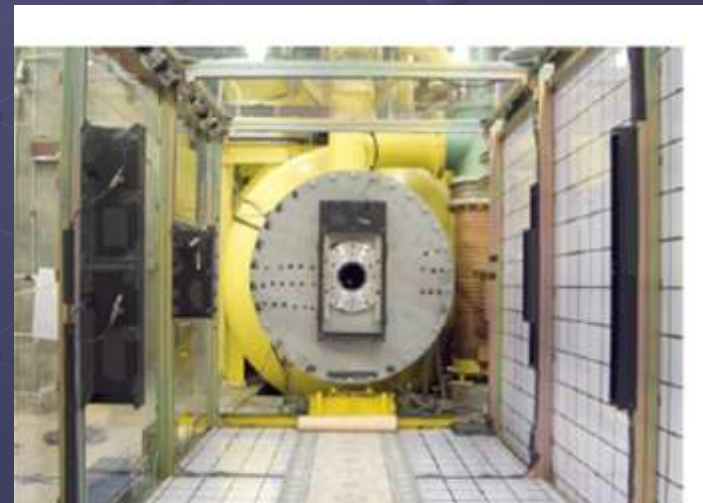
Test Section - Diaphragm, Lights, Light Screens, and Calibration Grids
