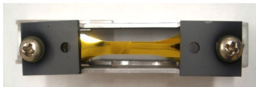
Figure 5.—Unstressed SiO x /Kapton HN sample AO-U-2 post exposure on MISSE 6.
