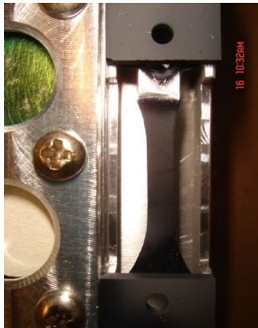
Figure 11.—Kapton XC flown on ram side of MISSE 6 (AO-S-1) showing stretching of sample at silvered area at the top.
