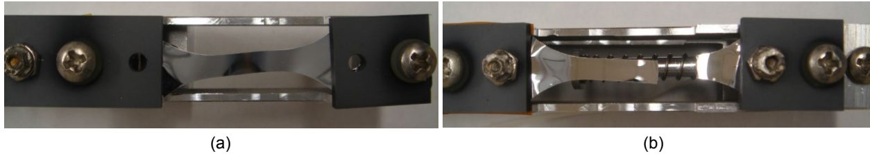
Figure 9.—(a) Unstressed VDA/CP1 sample AO-U-7 flown on the ram facing side of MISSE 6. (b) Stressed VDA/CP1 sample AO-S-5 flown on the ram facing side of MISSE 6. Sample broke sometime during the exposure on ISS.
