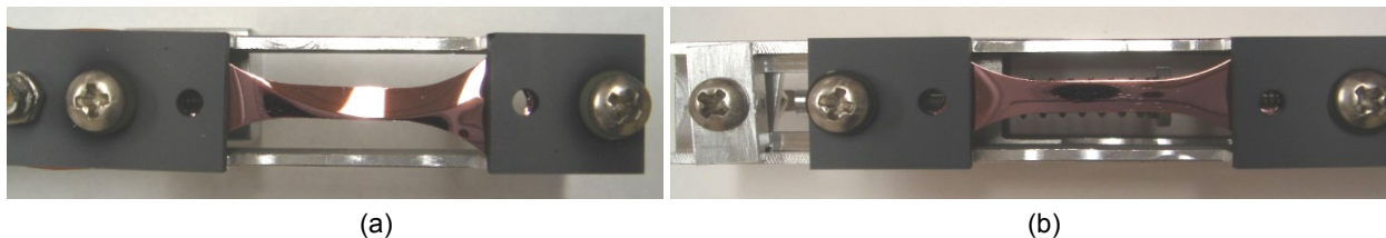
Figure 8.—(a) Si/Kapton E/VDA/Inconel/VDA sample AO-U-4 exposed on ram side of MISSE 6 unstressed. (b) Si/Kapton E/VDA/Inconel/VDA sample UV-S-4 exposed on wake side of MISSE 6 under stress showing some evidence of coating cracking
