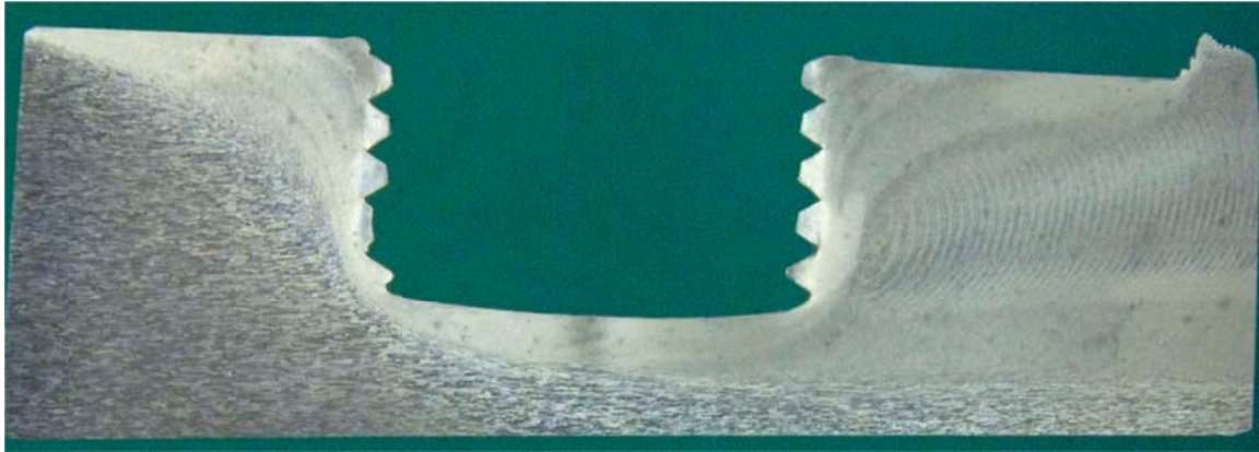
Figure 6. Formation of “tool marks” and internal banding. Lateral section of conventional friction stir weld cavity in 5 mm thick 2195-T6 aluminum alloy courtesy of J. McClure, University of Texas at El Paso. The lead angle of the tool is 3^\circ . “Tool marks” emerge from trailing edge of shoulder at right where the shear surface encounters the crown surface. Bands emerge from lower portion of shear surface where the ring vortex flow is outward. Bands do not emerge from the upper region of the trailing shear surface where the ring vortex flow is inward.
