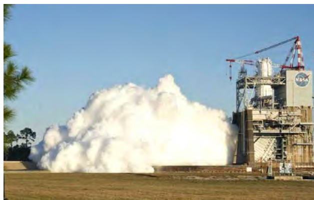
First J-2X Stability Test: 80-sec duration test firing; NASA began characterizing the rocket engine's combustion stability
