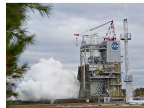
J-2X 500-sec test firing at SSC
